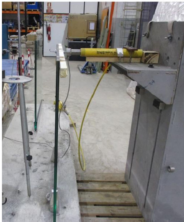
Appearance after horizontal outward push
